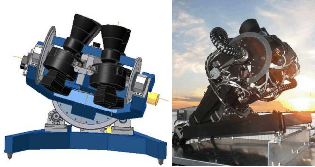
Figure 4. Detector unit of the final “Pi of the Sky” system: mount design (left) and the picture of the first detector unit installed in the INTA El Arenosillo test centre near Huelva, Spain, (right).
