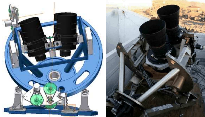
Figure 1. “Pi of the Sky” prototype at Las Campanas Observatory in Chile: 2004 mount design (left) and picture of the mount with Canon lenses used from May 2006 (right).
